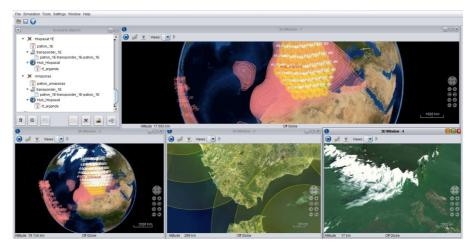
This software allows designing Satellite Contours and Service Areas for reporting ITU. GeoBeam is fully compatible with ITU software such as GIMS. It also allows the Satellite Operator to analyze and calculate with the designed coverage contours before presenting them for ITU approval. This is an easy check which makes a big difference fulfilling the ITU requirements.
