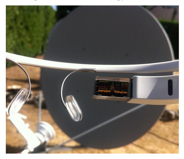
As the first Google Glass App especially design for the Satellite Industry, Satmotion Pocket opens the door to final customer VSAT installation; and now with Google Glass both hands are free for antenna alignment purposes, allowing the installer to look at the critical line up parameters in the most extreme weather conditions.
